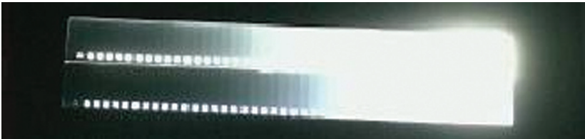
Test scene with over 90dB of dynamic range – SureVision (on the bottom) demonstrates far more dynamic range in this test scene.
